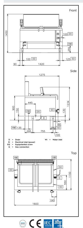
**Electric** Supply voltage: 291161 (CR42G) 230 V/1N ph/50 Hz Gas Gas Power: 60 kW Gas Type Option: LPG; Natural Gas Gas Inlet: 1"1/4 **Key Information:** Number of wells: 2 Usable well dimensions (width): 625 mm Usable well dimensions (height): 410 mm Usable well dimensions (depth): 640 mm 190 It MIN; 190 It MAX Well capacity: External dimensions, Width: 1600 mm External dimensions, Depth: 1280 mm External dimensions, Height: 850 mm Net weight: 386 kg
